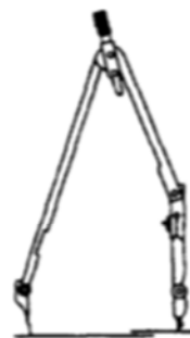
(b) Position of the lead leg to draw larger circles
