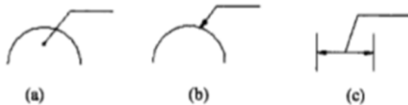
Fig. 2.21 Termination of leader lines
